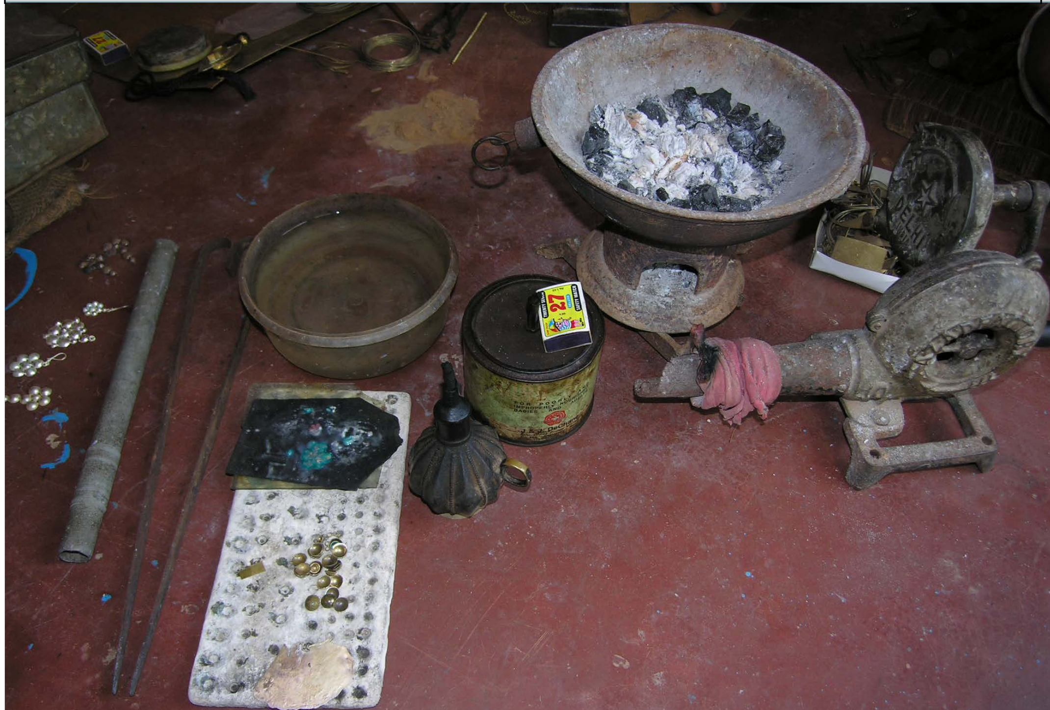
From left to right - metal pipe to blow air into the fire, tongs (chimuta) used to hold pieces of burning coal as well as other things, bowl of water, asbestos sheets used to place the metal pieces for welding, small glass sheet holding the soldering material which is made of pure silver leaf (nisha jhal, khar or tanganu), water, Kerosene lamp for the fire (Dibbir), iron stove (Umaei), blower (Bhathi)
