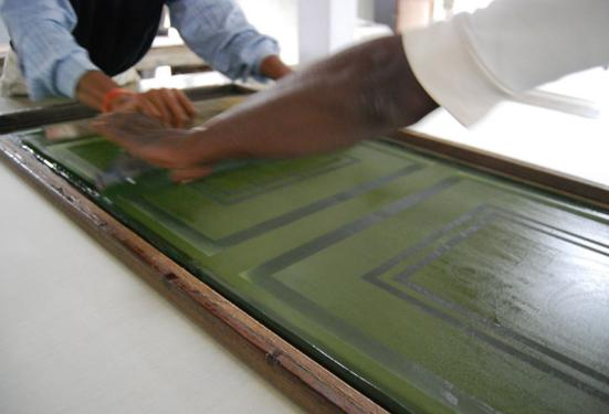
screen – a frame of a very thin filament with the designs printed on it – is aligned on the fabric.
