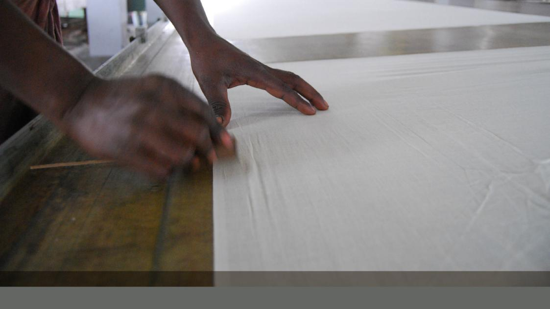
The field of cloth is stretched and pinned on the block-printing table in the porch outside.
