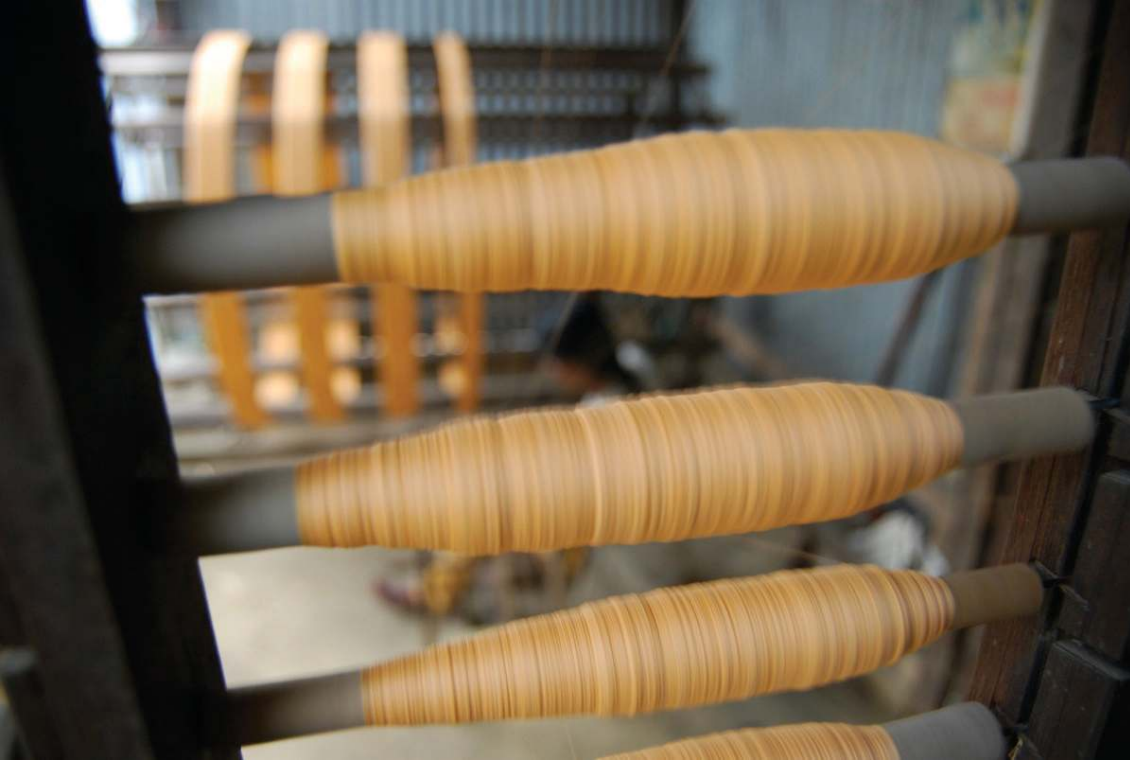
From bobbins, the yarn is transferred on to large drums, a process called 'drumming'.
